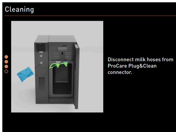
Figure: Removing milk hoses from Plug&Clean connections
