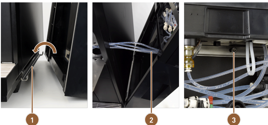
Figure: Fastening ProCare unit to machine
