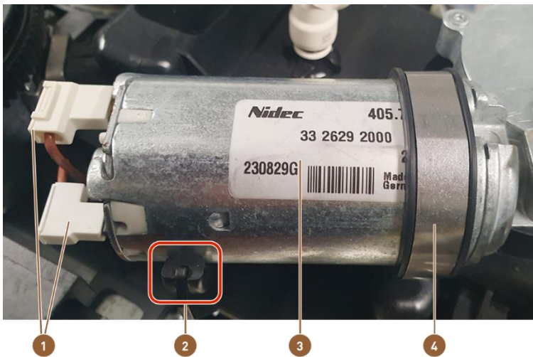
Figure 1: Brewing motor with previous cable grommet 3370013550
