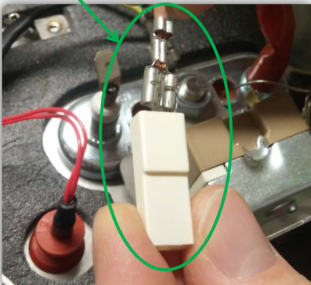
12. Put the cover on the female faston
