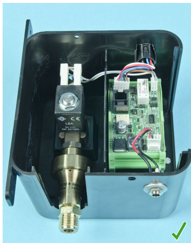
Connection housing with new electronics
