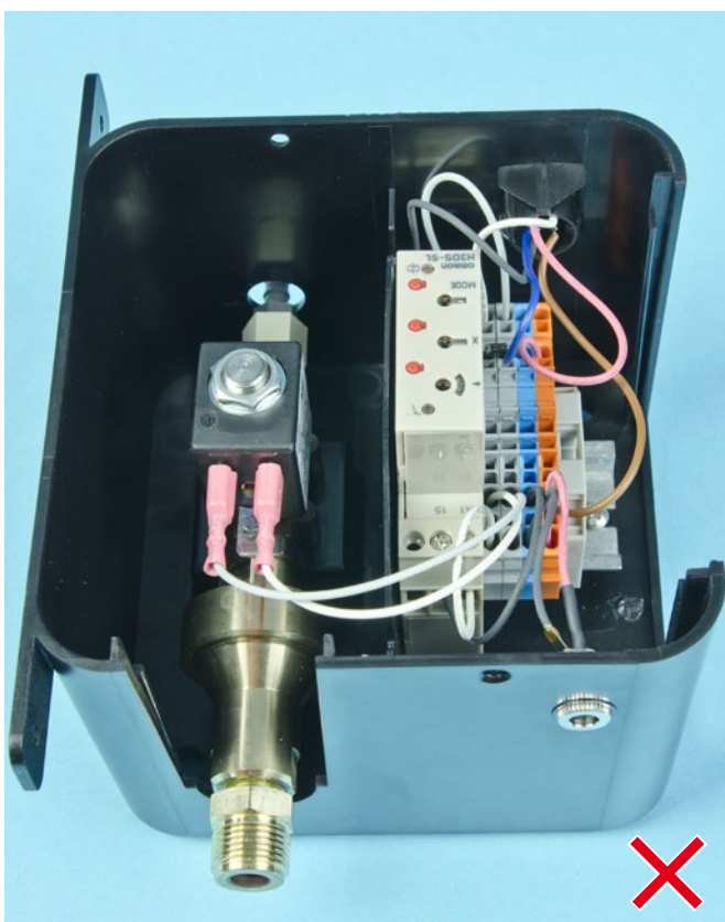
Connection housing with old electronics
