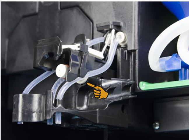
Beverage outlet without cover hood, side view. Correct positioning of the steam nozzle.
