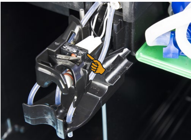
Beverage outlet without cover hood, view from top. Correct positioning of the microswitch.
