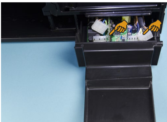
Removing the integrated power supply insert.
