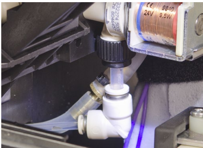
Relief pipes once installed
