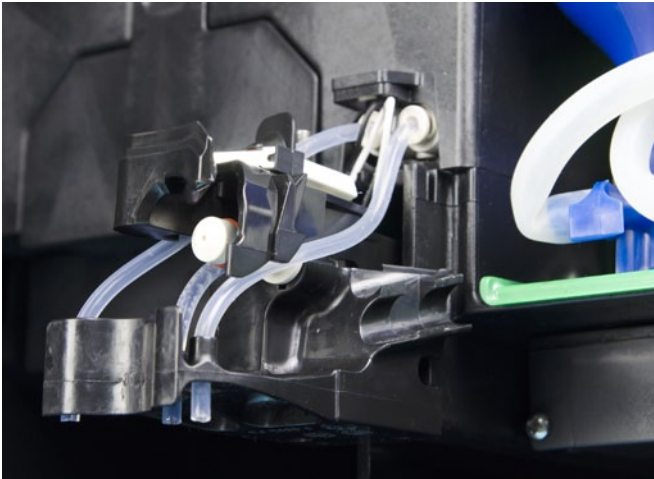
Beverage outlet without cover hood, side view.
