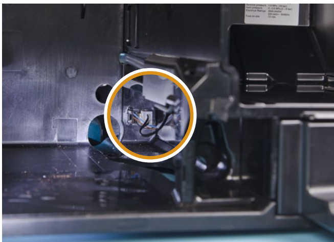
Disconnecting the sensor plugs.
