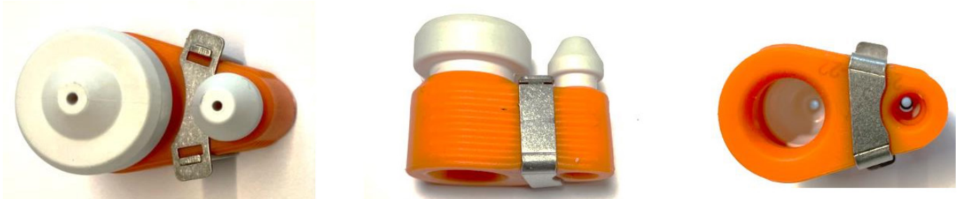
Figure 2: Metal clip taking the example of an orange suction chamber
