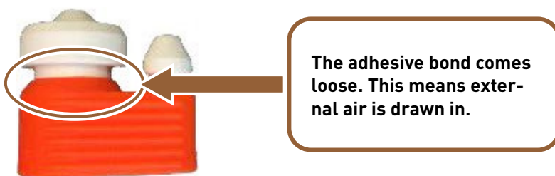
Figure 1: Adhesive bond between nozzle insert and elastomer element
