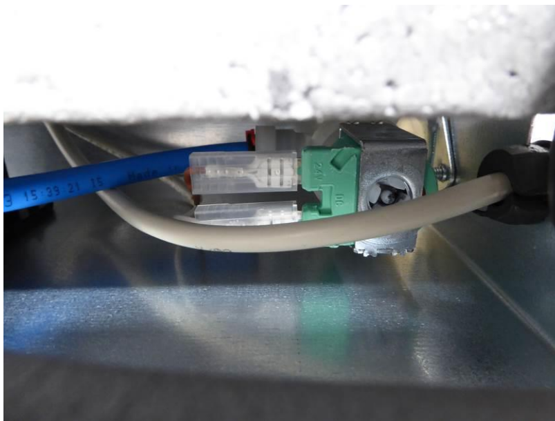
Water valve in position
