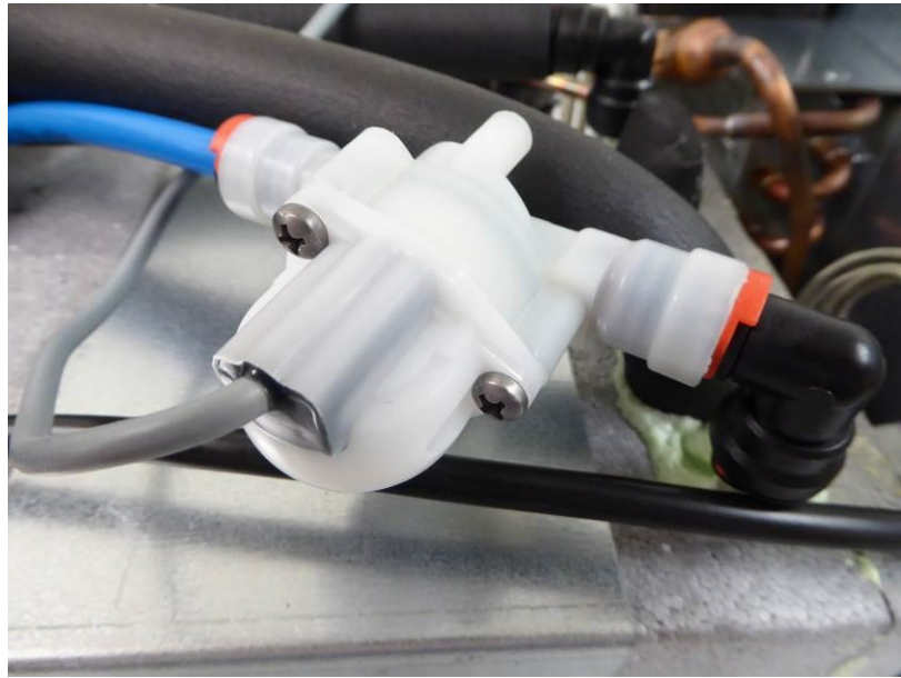
Flowmeter in position
